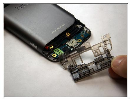
Once the screws are removed from the plastic flap, the piece should easily come out.
