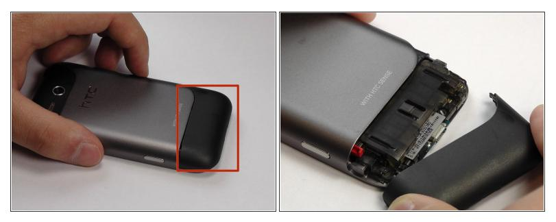
• Apply pressure to the dark plastic casing and slide the casing downward, off of the phone.
