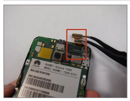
• There are two more ribbon cables at the top that must also be disconnected, to do this simply lift them up from their connecter with the tweezers or with the spudger.
