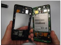
Use the plastic opening tool by fitting it into the gaps to pull back the frame.
