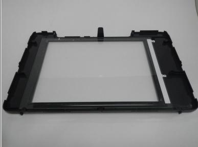
Lift the scanner glass piece from the printer and set it aside.
