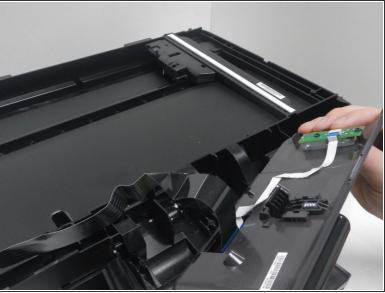
Place thumb and forefinger where shown and pull this piece away from the printer.
