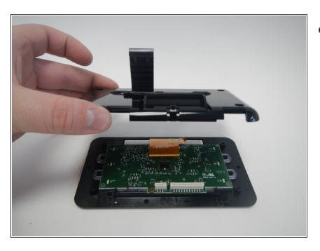
Lift the back of the display screen to remove it.
