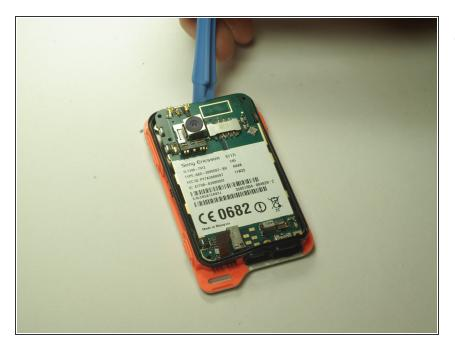
Using the plastic opening tool, carefully pry up on the edges of the motherboard, opposite of the jacks.
