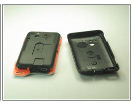
• Open the flaps and remove the back cover using the plastic opening device.
