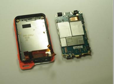
• Carefully pry up on the tab holding down the display ribbon cable and remove the ribbon cable.
