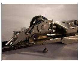
Unscrew the screw located underneath fork arm using a Flathead screwdriver.
