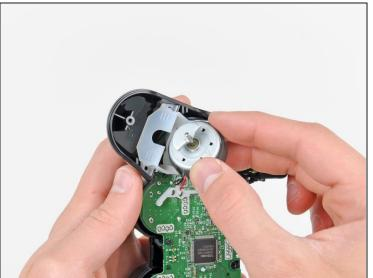
• Pull the vibration motor out of its plastic frame, being careful not to strain the wires connecting it to the motherboard.
