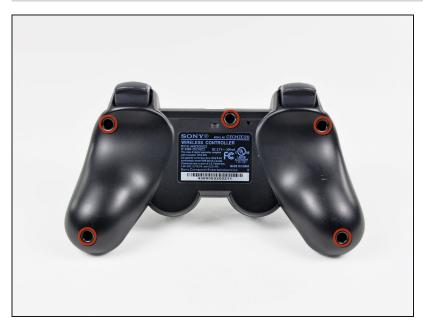
• Remove the five 7.2 mm Phillips screws securing the rear cover to the controller.
