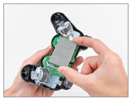
Lift the battery off the motherboard for enough clearance to access the battery connector.
