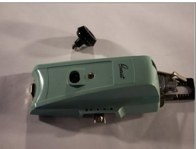
Press down on the adjusting knob, and turn it to the left until the knob is unscrewed.
