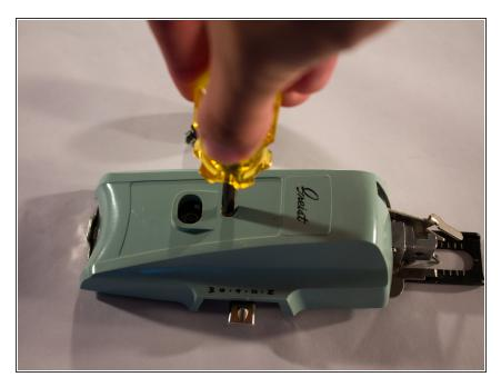
Using the phillips screwdriver, unscrew the cover screw.
