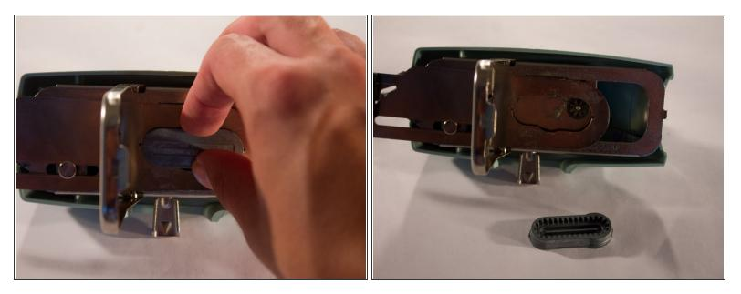
• Since the clamp is extended as far as it can go, the template should come out easily.
