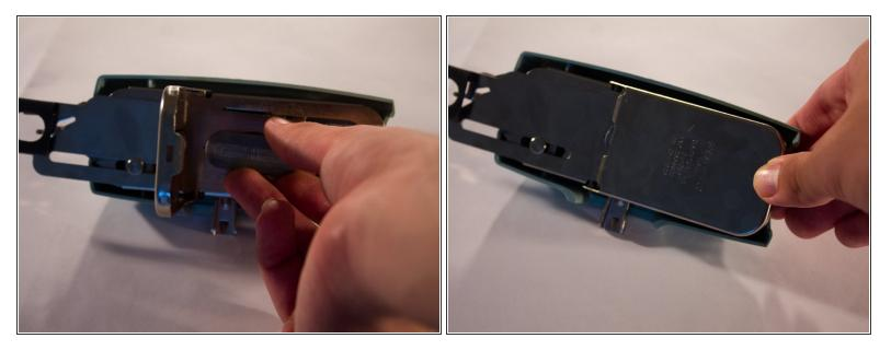
• Place the template into The Buttonholer, and then close the retainer plate.
