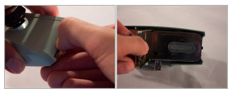
Located on the bottom, pull the lip of the retainer plate away from The Buttonholer, and then open the plate.
