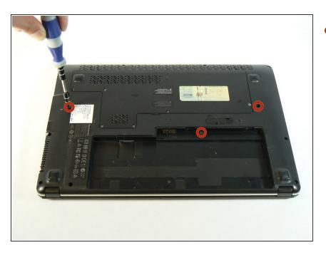
Unscrew the three screws on the bottom of the laptop that have small keyboard logos next to them using a PH1 screwdriver. These screws are 5.8mm long.
