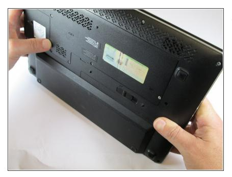
• Locate the battery by turning the laptop over.
