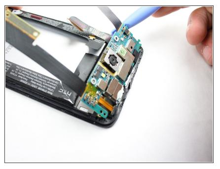
Slowly lift the camera board up and work on removing the remaining adhesive. You can then take the camera board off of the phone.
