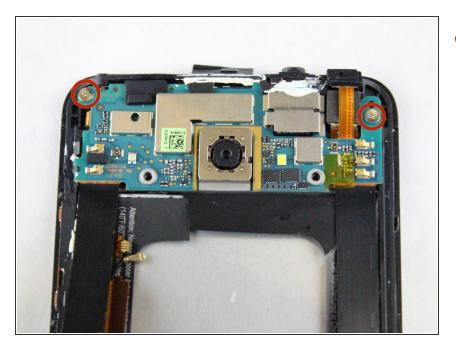
Use a Phillips #000 screwdriver to remove the two 2.1mm screws on the top of the camera board.
