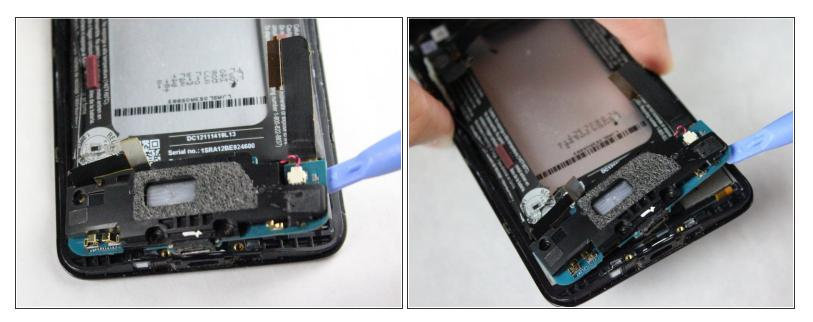
• Use the plastic prying tool to gently remove the charging port assembly.
