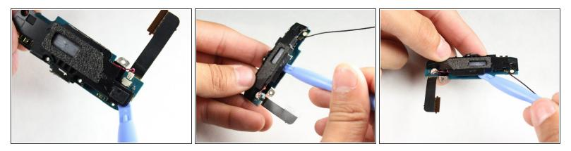
• Use the plastic prying tool to separate the assembly into two pieces: blue and black.
