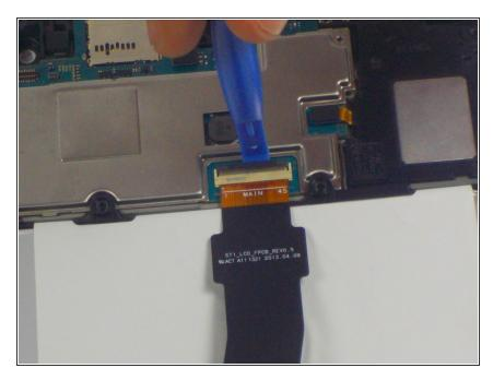
Gently remove tape over ribbon cable connectors and set it to the side. Using the opening tools, gently lift the connector latches to disconnect the ribbon cables.
