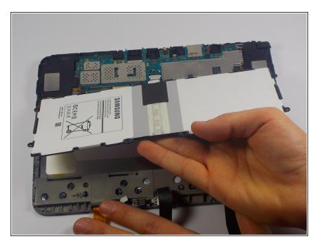
Pull back the ribbon cables, lift up the original battery, and disconnect the battery by exerting upward pressure from beneath the battery.
