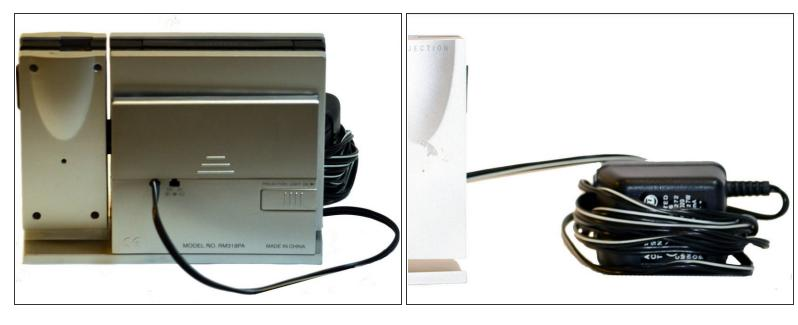
To access the A/C Power Adapter connection, remove the battery cover, located on the back of the clock.
