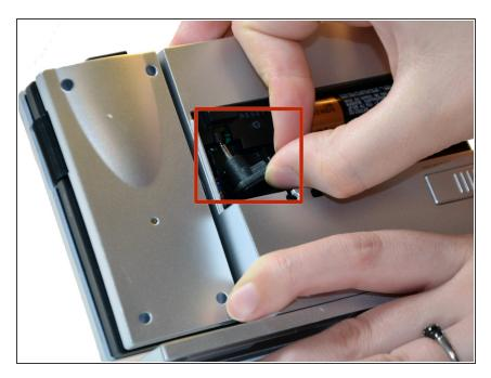
Gently pull the A/C Power Adapter from the socket, to the left of the batteries.
