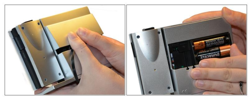
To remove the battery compartment cover, slide the cover up towards the top of the clock while applying slight pressure.
