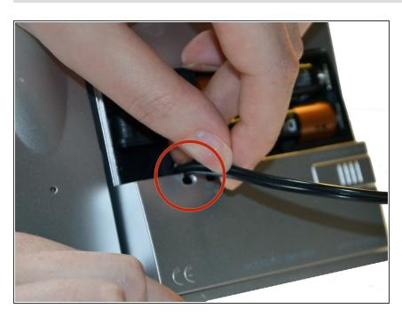
Once the A/C Power Adapter tip is inserted in the socket, guide the cord through a notch directly below.
