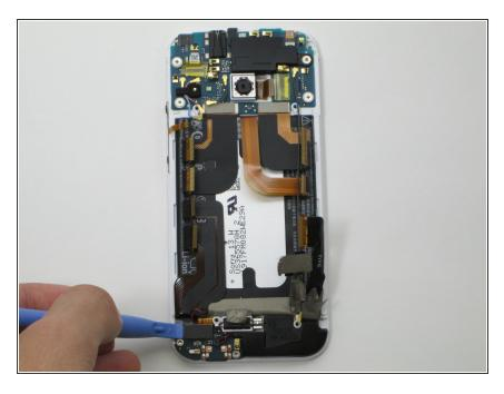
Using the narrow plastic prying tool, pry up the rectangle connector covered in black foam
