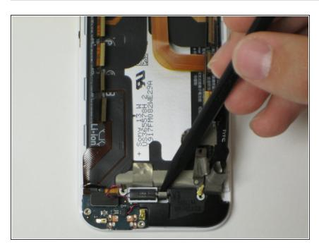
Use the pointed end of the spudger to pop the rumble motor out of its housing.
