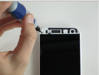
Remove the 2mm screw with a T5 torx screwdriver head from the iFixit tool kit.
