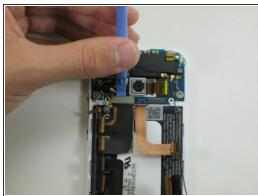
Use the narrow plastic pry tool to pop off the two ribbon cable connectors located at the bottom of the upper circuit board.
