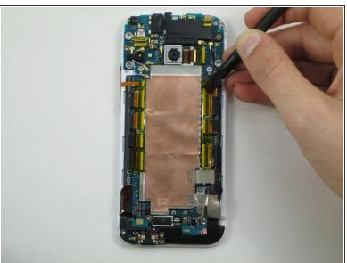
Peel off the long yellow pieces of tape on the right and left side of the copper plate.
