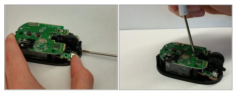
Using prying tool press against the bottom of each side of the click wheel apparatus to cause it to snap out of place.
