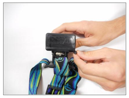
Remove the back cover of the battery housing (found behind the mount assembly) by pulling the small tab on the bottom right corner.
