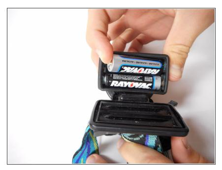
Remove the old batteries by pulling outward the positive end of each battery.
