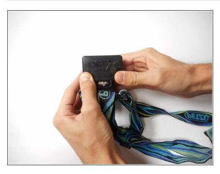
Reattach the back cover of the battery housing by pushing in the bottom half and then pressing the rest of the cover into place.
