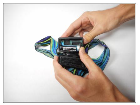
Insert the new batteries by inserting the negative end of the battery into the negative side of the battery compartment and pushing the positive end of the battery into the positive side of battery compartment.
