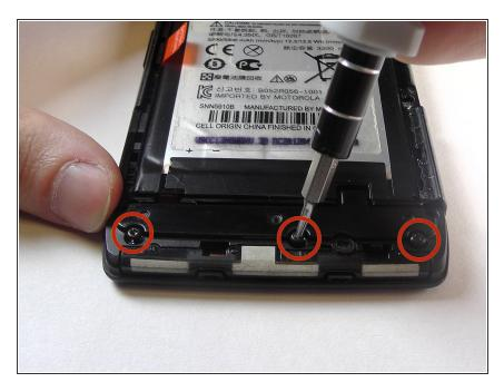
Using the T5 bit piece remove the three black 4.5 mm screws that are located at the bottom of the phone.
