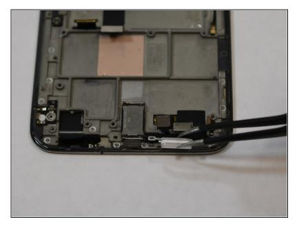
After the plastic plate is removed, <u>tweezers</u> can be used to remove and replace the power and volume buttons from the device.
