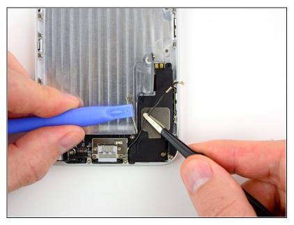
i To fully de-route the antenna connector, you may need to gently pull back the metal clip securing it to the speaker assembly.
