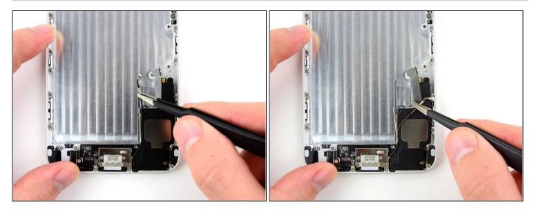
• Grasp the antenna connector with a pair of <u>tweezers</u> and carefully begin de-routing it from its channel on the speaker.
