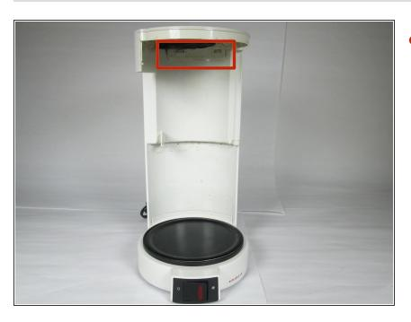
Locate the two plastic latches on the inside of the coffee maker.
