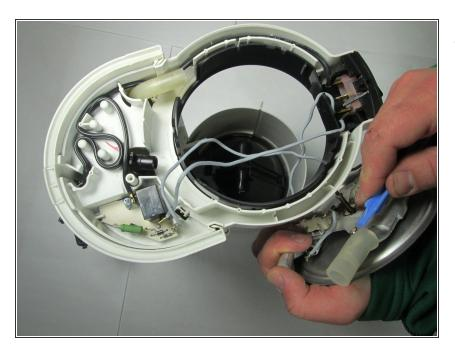
Using the larger plastic opening tool, gently push the tubing off of the center plate. (If the tubing is being stubborn and won't come off, run the metal spudger around the inside of tubing to free it up.)
