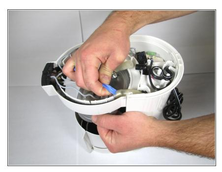
Using the larger plastic opening tool, gently push the tubing off of the valve located on the side. (If the tubing is being stubborn and won't come off, run the Spudger tool around the inside of tubing to free it up.)
