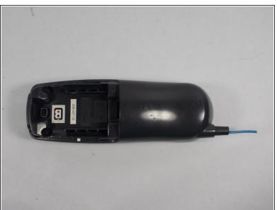
Your first step will be to remove the battery cover and the battery.
