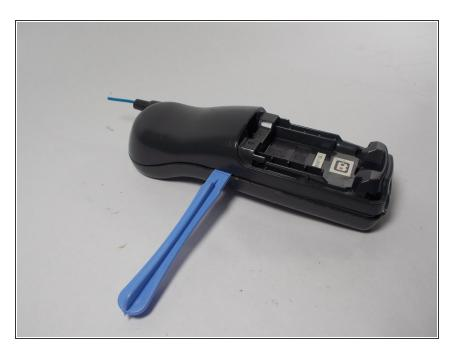
After that you will need to pry the back of the case off of the front part of the case.
