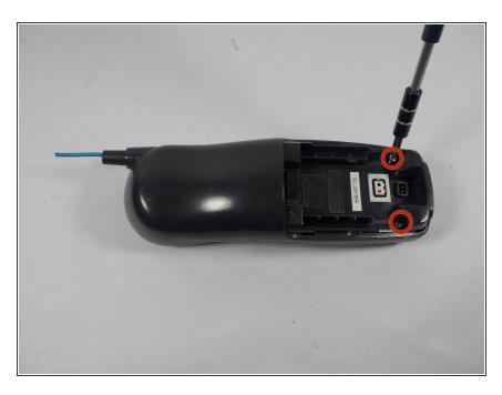
The next step will be to remove the two screws from the rear of the phone case.
