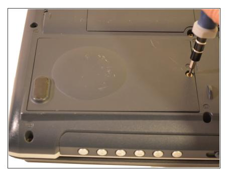
Unscrew the single small screw labeled F4 located on the right side of the panel.
