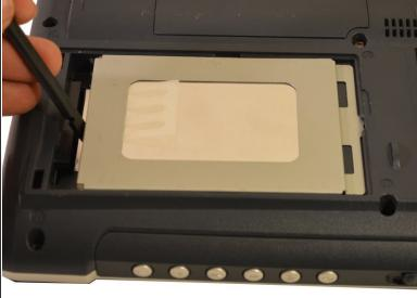
• Use a spudger to disconnect the hard drive by shifting the entire drive to the right.
