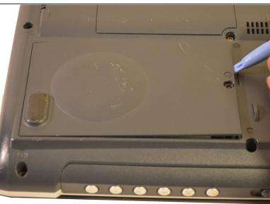
Insert a spudger into the indent near the screw to pry open and remove the cover.
