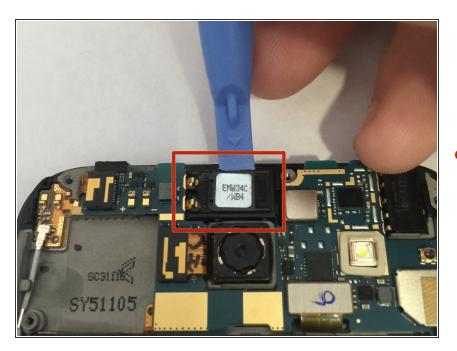
Once you have completed the prerequisites, the speaker should be accessible for removal. Using one of
