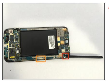
The logic board is connected to the under side of the phone with a bit of adhesive. Using a spudger, place it under the logic board from the top right corner and gently slide it toward the center orange mark where the adhesive is. Apply a little bit of pressure parallel to the logic board and the Logic board should loosen from the phone.
