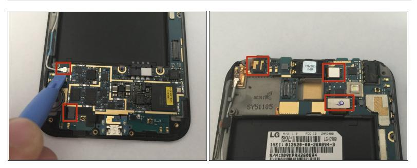
Use the plastic opening tool to disconnect the 4 ribbon cable connections and the antenna attached to the logic board.
