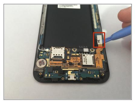
Using your plastic opening tool, disconnect the connection between the phone and the ribbon cable.
