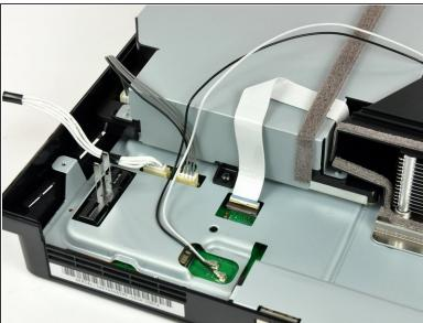
(i) If present, remove the pieces of tape securing the cables to the body of the Blu-ray drive.
