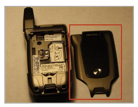
Reattach back cover and secure all components in place.
