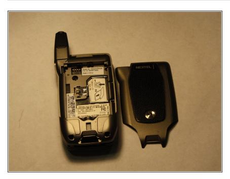
Remove back cover of the phone by disengaging the clip and lifting up on the cover.
