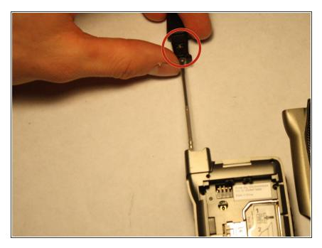
Slide and secure new antenna into position. Make sure metal receiver is facing forward.
