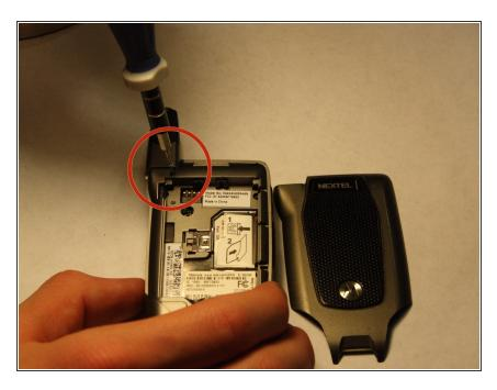
Locate the screw on the top left portion of the phone; just below the antenna. Using a T4 Torx screwdriver remove the screw.
