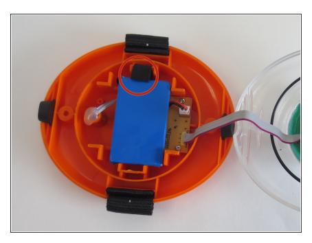
Seat the battery in the orange component so that the short end of the battery pack is touching the foam bumper.
