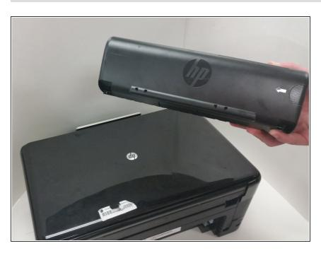
The duplexer is now removed from the printer.
