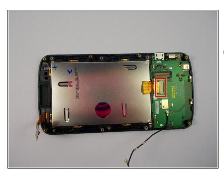
Unlock the ribbon cable and then you can pull the screen out.
