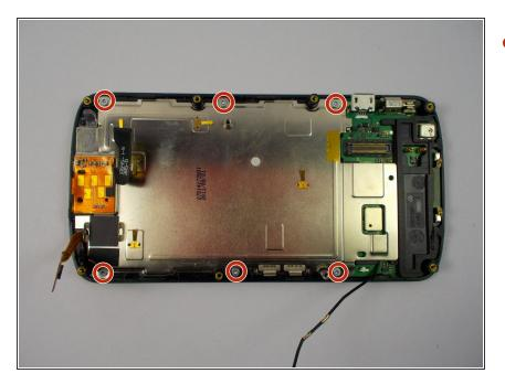
Unscrew the 6 screws using the T5 Torx screwdriver.
