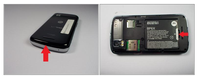
Remove the back cover and battery by using the thumb tabs.
