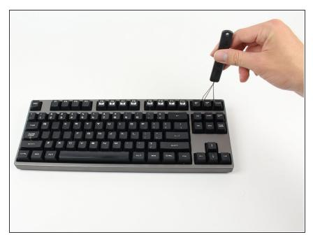
Insert the keycap puller around the key you'd like to install an O-ring under.
