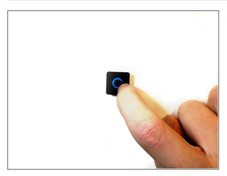
Place an O-ring around the plastic shaft located on the underside of the keycap.
