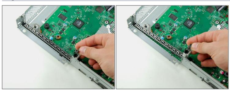
Lift the optical drive retaining bracket off the logic board.
