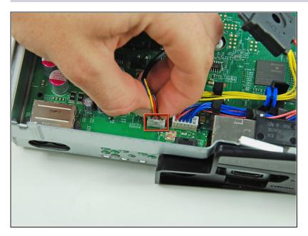
Disconnect the fan cable by pulling its connector off the logic board.
