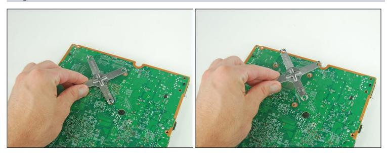
• Lift the x-clamp off the back of the logic board.
