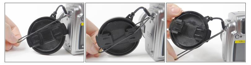
Separate the two pieces of the loop and pull the lens cover up in between them.
