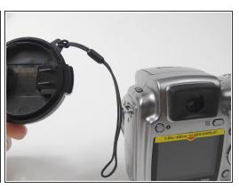
Pull the lens cover and the sting will come out of the metal slab.
