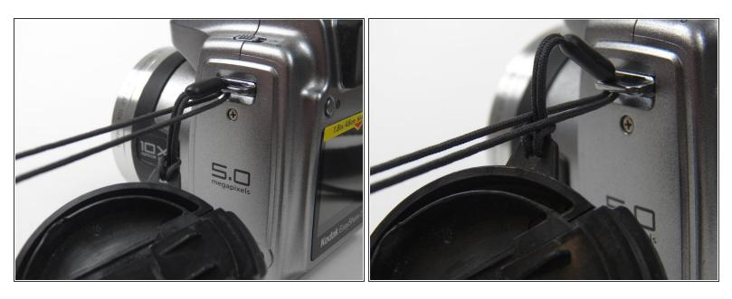
Feed the string on top into the metal slab while pulling the loop toward you until the plastic piece stops you from pulling any further.
