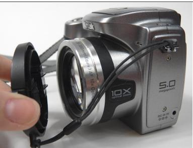
Remove lens cover from the camera by squeezing the protruding button on each side of the cover and pulling.
