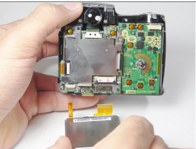
Gently pull the LCD screen down until the orange cables separate from the motherboard.
