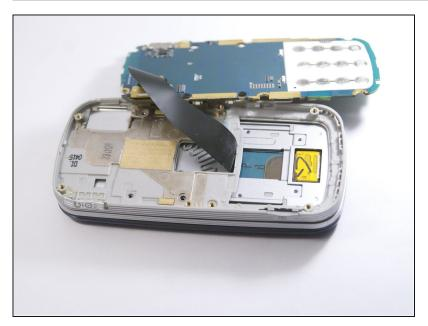
Carefully lift up to motherboard to expose the power button.
