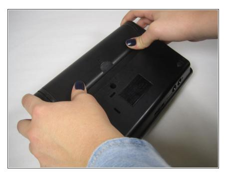
• Use your thumbs to press firmly down and then push the battery door cover open.
