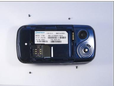
Use a Phillips screwdriver to remove the four 2mm Phillips #000 screws from each corner of the device.
