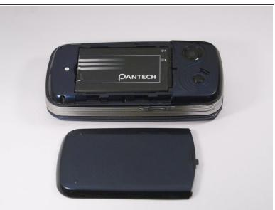
Gently slide the backside phone cover off exposing the battery underneath.
