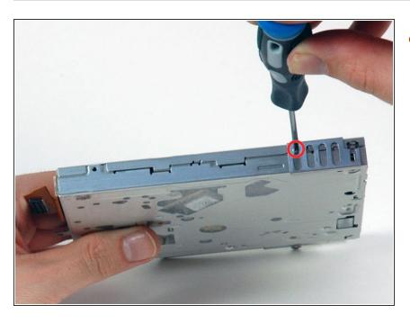
Remove the single Phillips screw securing the mounting bracket to the left side of the optical drive.
