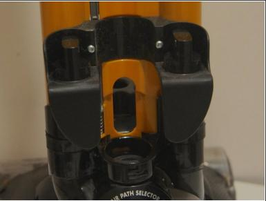
Grasp the thick smooth collar at the bottom of the hose and twist left (counterclockwise) to remove the hose. To reassemble your device, follow these instructions in reverse order.
