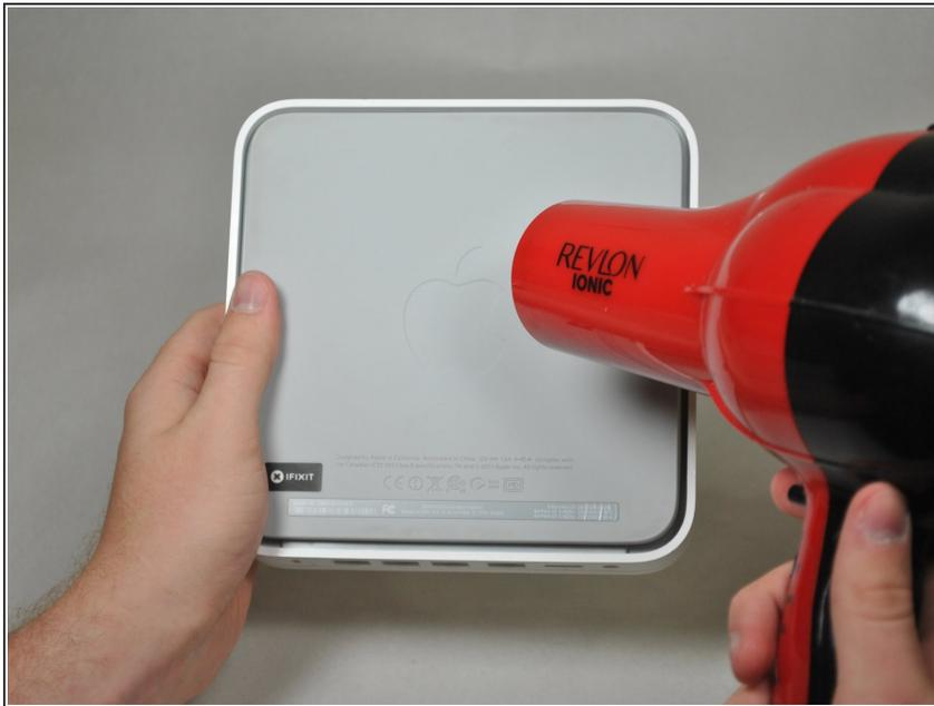
**⚠ CAUTION:** The heat gun and hair dryer can get very hot. Do not put your hands or any other body part too close to either device. Also, do not touch the back pad right after heating it.
