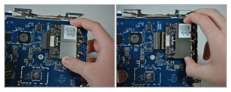
⚠ Do not pull the WiFi card directly up or you may damage the slot and the logic board.
