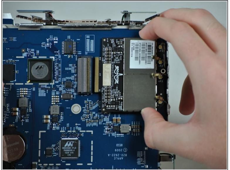
**⚠ Do not pull the WiFi card directly up or you may damage the slot and the logic board.**
