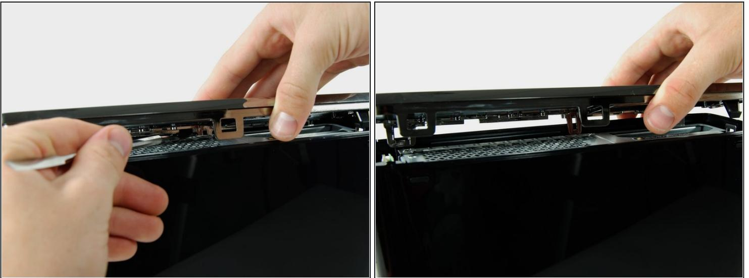
ⓘ This clip is smaller than the others and should not be removed from above like the others.
