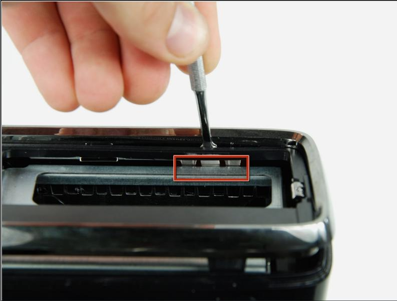
ⓘ This clip does not have a slit in the bezel to guide you. You can locate the clip by looking under the bezel near the hard drive slot.
