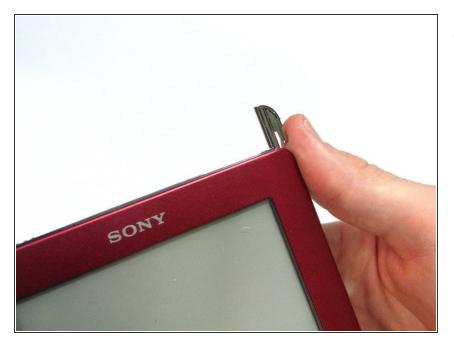
Remove the stylus from the device.
