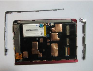
Pull the panel away from the device. You may have to use the flat end of the spudger to remove the side portion of the panel because it will be glued in place.
