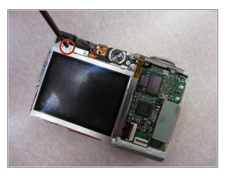
Unscrew one .113 inch Phillips screw using a #00 Phillips screwdriver.
