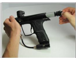
Using the 1/4" hex key, turn the bolt counterclockwise and remove.
