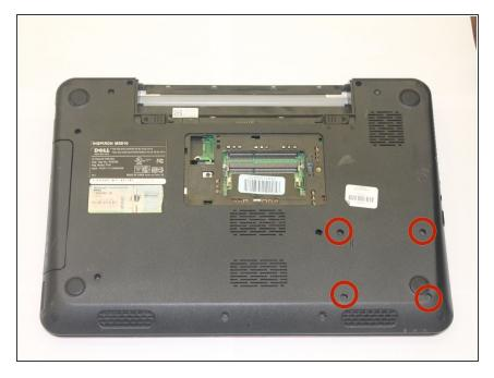
Remove the 4 mm Hard Drive screws with the Phillips #000 screwdriver.
