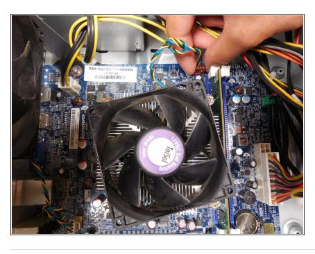
Unplug the fan from the motherboard by gently pulling out the single plug. Then lift the fan up and out of the computer.
