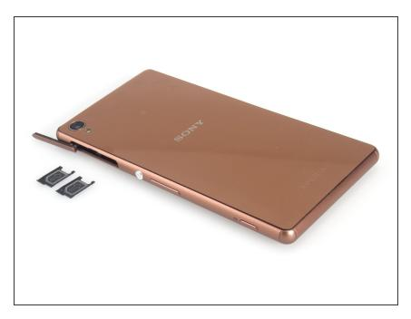
Power off the phone and remove two SIM card trays before replacement.
