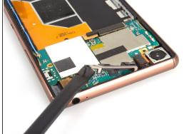
Remove three pieces of securing bracket.
