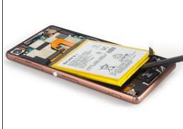
Remove battery or not is optional. Remove it makes the replacement convenient while keep it also will not block the replacement.
