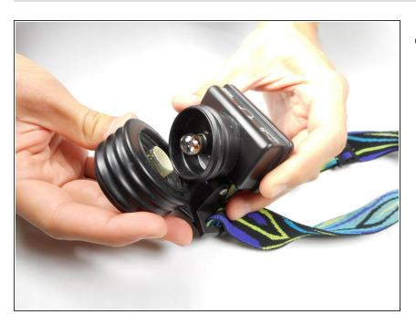
Remove the lens piece by firmly pulling it away from the battery housing.
