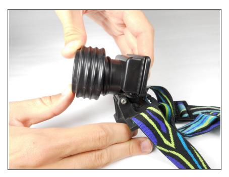
Press the lens piece onto the front of the battery housing.
