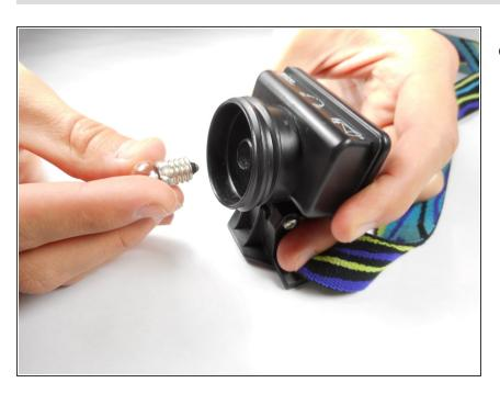
Install the new bulb by inserting it into the socket.
