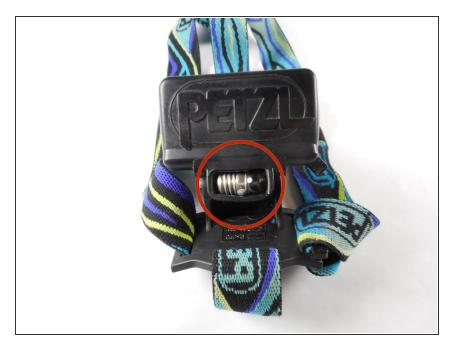
Check for a spare bulb in the spare bulb compartment located on the back of the battery housing (found behind the mount assembly). If no spare bulb is found in the spare bulb compartment you will need to purchase a replacement 3V incandescent bulb from a reputable retailer
