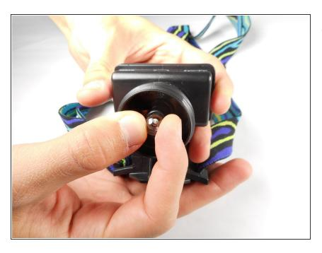
Rotate the bulb clockwise (right) until it is firmly fixed in place.
