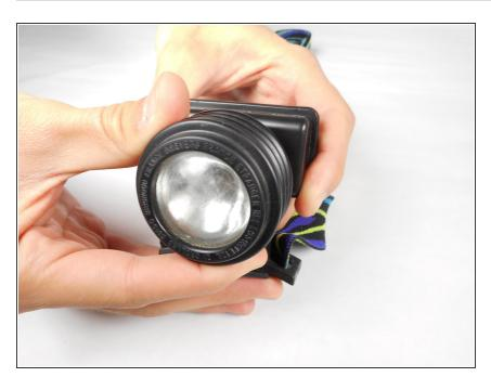
Turn the lens piece counterclockwise (left) until it is fully extended.
