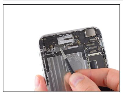
Grasp the antenna bracket with a pair of <u>tweezers</u> and lift it off the iPhone.
