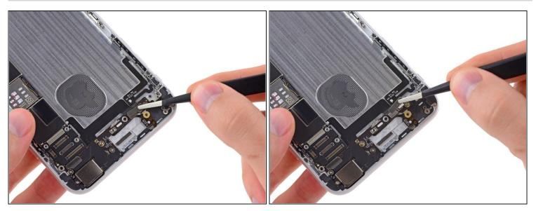
• Use a pair of <u>tweezers</u> to peel the single adhesive tab that resides on top of both the power button and audio control/rocker switch cable connectors.
