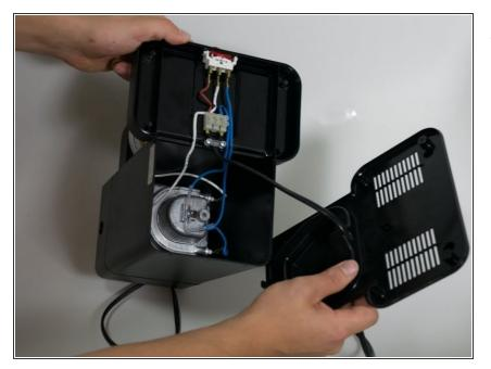
Remove the bottom cover from the machine and slide it down the power cord.
