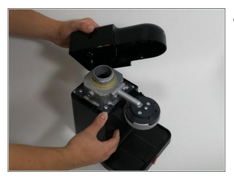
• Lift and remove the top black plastic cover from the machine.
